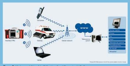
Figure 2: Wireless capabilities of the Philips HeartStart MRx monitor/defibrillator.
