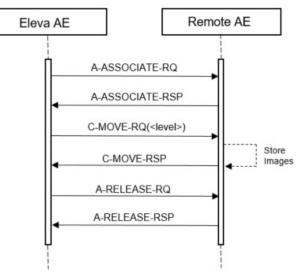
Figure 13: Data Flow Diagram – MOVE as SCU
