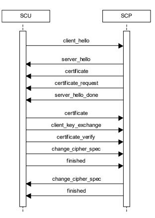
Figure 17: Message flow of TLS handshake
