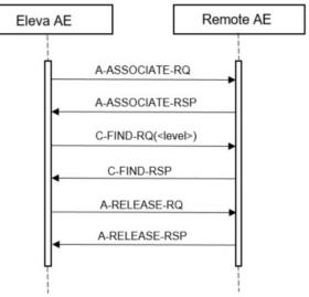
Figure 12 Data Flow Diagram – FIND as SCU
