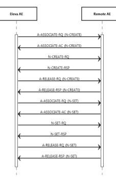
Figure 7: Modality Performed Procedure Step as SCU
