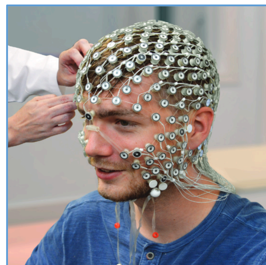
Figure 2. Whole head sensor net distribution of 256 electrodes.
