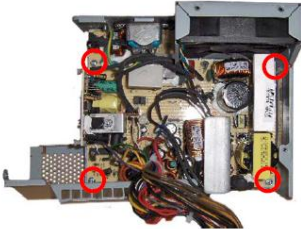
FIGURE 14: Power supply PCA screw locations
