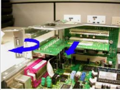
FIGURE 6: Removing the power USB and COM cards
