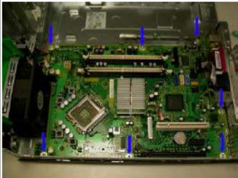
FIGURE 8: PCA screw hole locations
