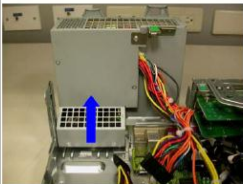
FIGURE 5: Removing the power supply
