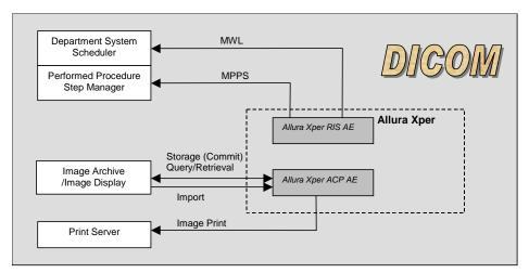
Figure 1 Data Flow of Allura Xper in a DICOM network
