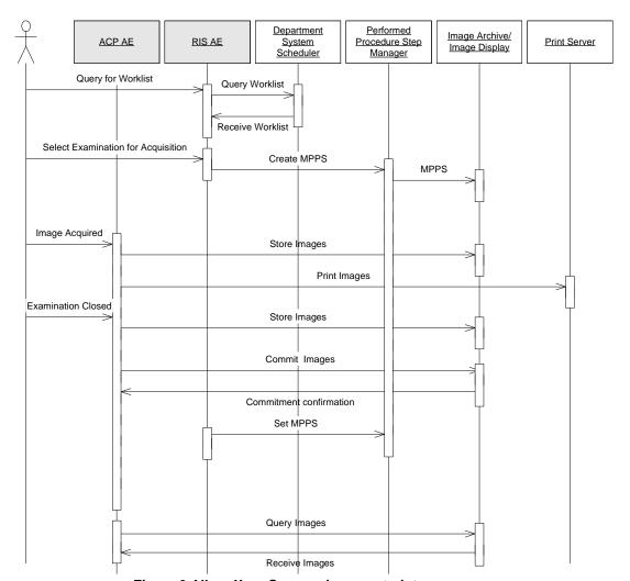
Figure 3 Allura Xper Sequencing constraints
