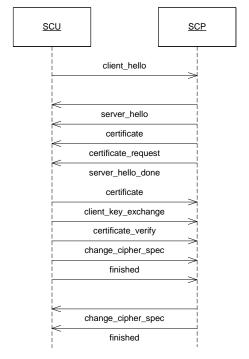
Figure 20 Message flow of TLS handshake
