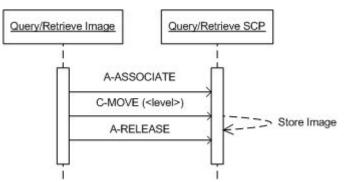
Figure 6: Data Flow Diagram - MOVE as SCU
