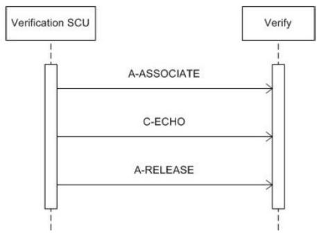
Figure 12: Data Flow Diagram - Verify
