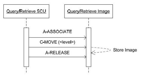
Figure 14: Data Flow Diagram - MOVE as SCP
