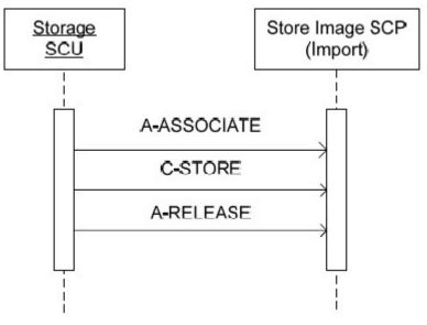
Figure 15: Data Flow Diagram – Store Image – Storage as SCP
