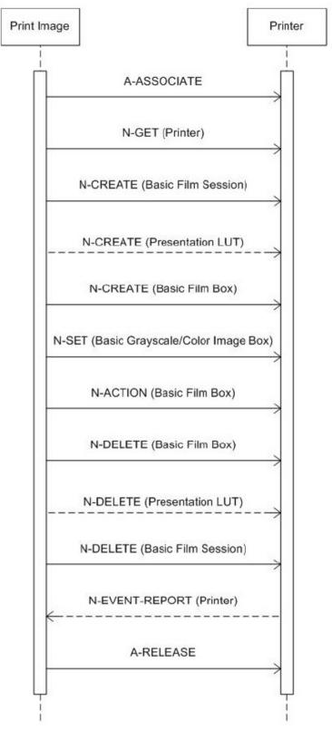
Figure 11: Data Flow Diagram – Print Management as SCU
