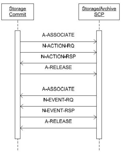
Figure 10: Data Flow Diagram – Commit Image (asynchronous)
