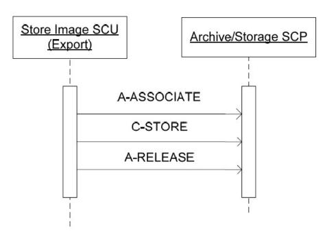
Figure 7: Data Flow Diagram - Store Image - Storage as SCU
