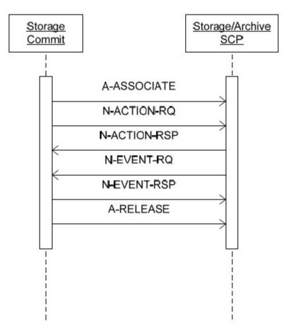
Figure 9: Data Flow Diagram – Commit Image (synchronous)
