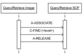
Figure 5: Data Flow Diagram - FIND as SCU
