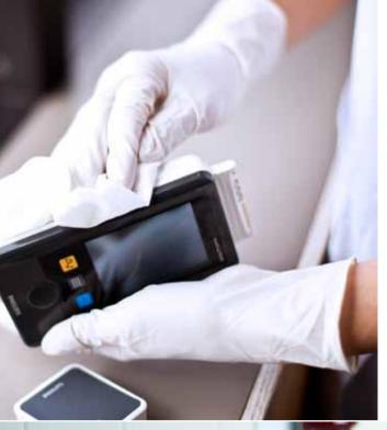
The IntelliVue MX40 is water tight (to IPX7) and able to withstand accidental water immersion, showering, and cleaning.
