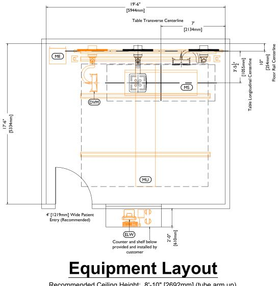
Recommended Ceiling Height: 8'-10" [2692mm] (tube arm up) or 10'-2" [3099mm] (tube arm down)
