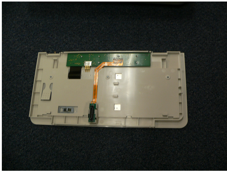
Figure3 circuit boards inside Cardiograph-keyboard PCA
