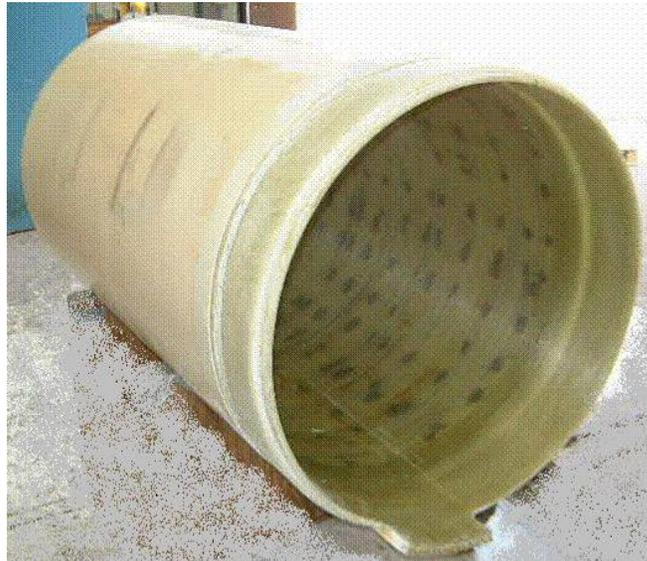
Figure 11 7T 3<sup>rd</sup> order shim tube, built with lead-free (silver) solder. Illustrated as removed from magnet.
