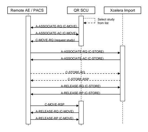
Figure 9: Flow diagram Retrieve DICOM image data from external DICOM node.
