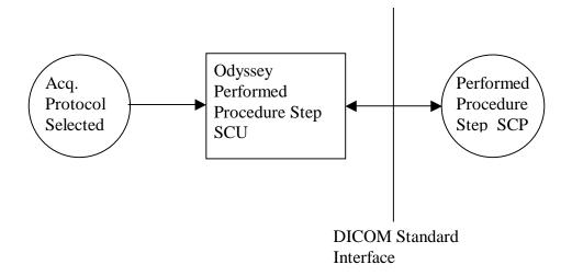
The Performed Procedure Step N-SET message is sent immediately after the acquisition has completed. If the operator aborted the acquisition, a DISCONTINUED status is sent, and no intervention by the operator is needed. In all other cases, the status that is sent is COMPLETED.
