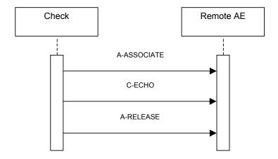
Figure 5. Sequencing of RWA Request Verification
