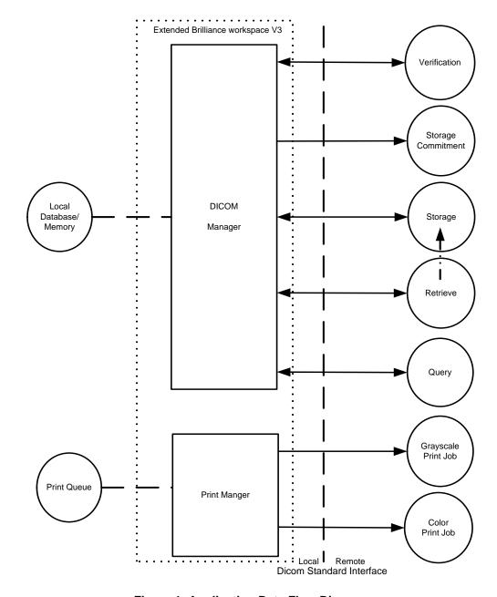
Figure 1: Application Data Flow Diagram
