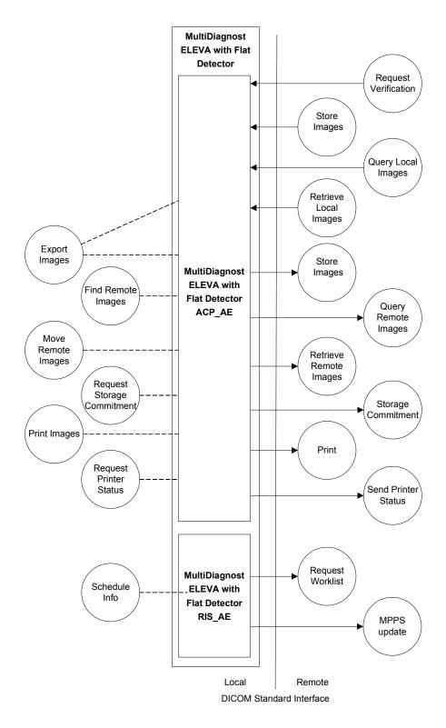
Figure 2: Networking Application Data Flow Diagram of the MultiDiagnost ELEVA with Flat Detector
