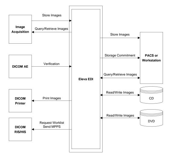
Figure 1: Eleva EDI MultiDiagnost R2 System in a DICOM Network environment
