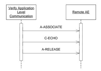
Figure 16 Sequencing of RWA Verify Application Level Communication
