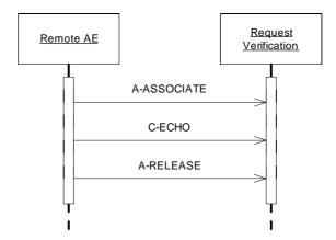
Figure 18 Sequencing of RWA Request Verification
