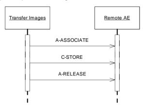
Figure 8 Sequencing of RWA Transfer Images
