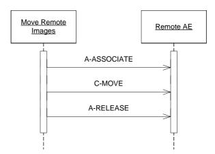
Figure 11 Sequencing of RWA Move Remote Images
