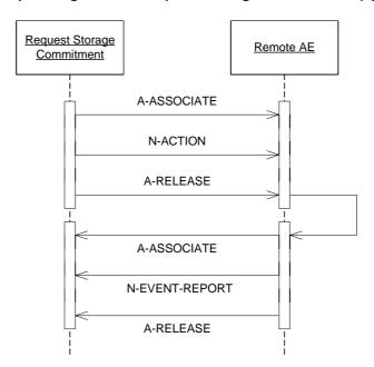
Figure 13 Sequencing of RWA Request Storage Commitment (asynchronous)
