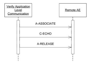
Figure 7 Sequencing of RWA Verify Application Level Communication
