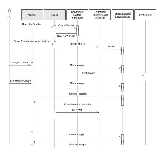
Figure 3 Allura Xper Sequencing constraints
