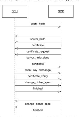
Figure 19 Message flow of TLS handshake
