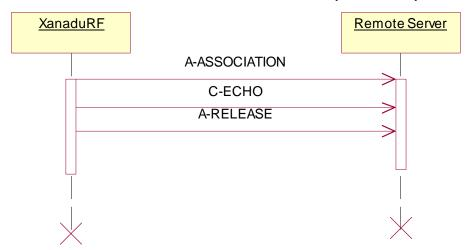
Figure 4-2: Sequencing of Verification
