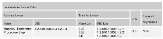
In the table the preferred transfer syntax is reduced sequentially from top to bottom.
