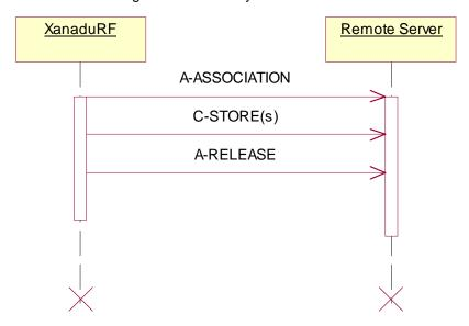
Figure 4-3: Sequencing of Storage Note:Storage and Storage Commitment are sepatate RWA's.
