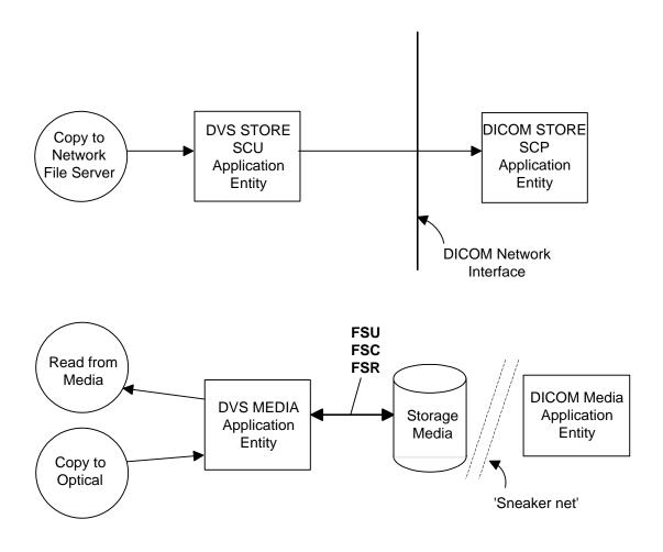
Figure 1-1 Real-World Relationships to Application Data Flow
