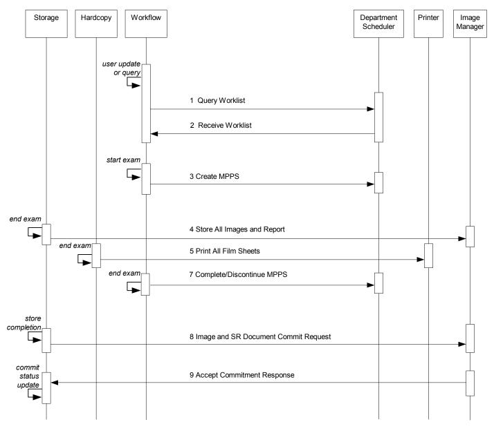
Figure 2b: SEQUENCING CONSTRAINTS – END EXAM CONFIGURATION
