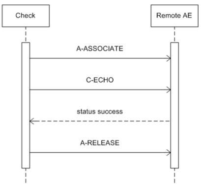
Figure 10: Sequencing of RWA Check
