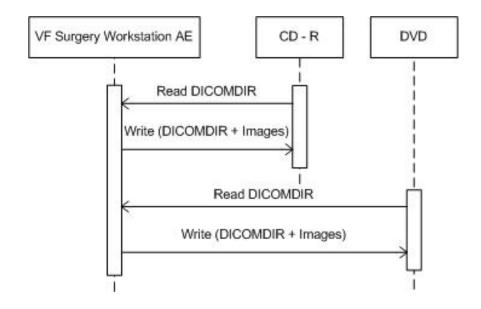
Figure 21: Sequencing of RWA Write Image
