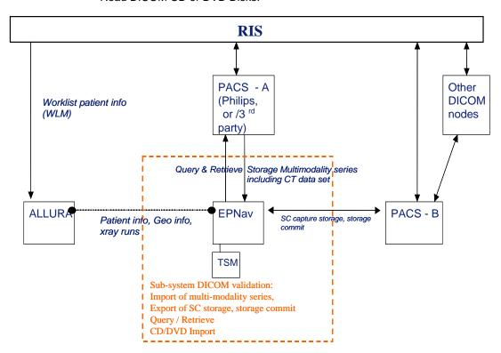
Figure 1: EP Navigator system context regarding DICOM connectivity interfaces
