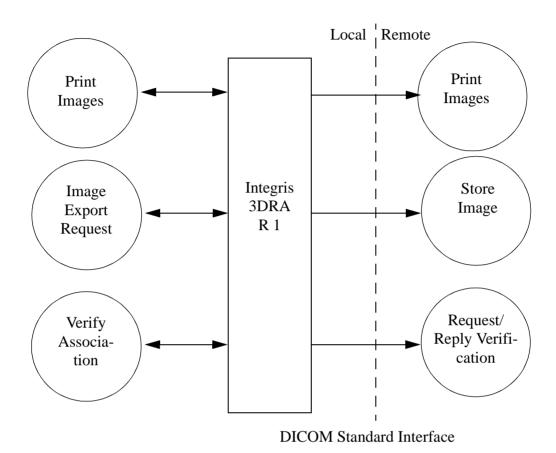
Figure 2-2: The Integris 3DRA DICOM Implementation Model (with references to the related sections. Within the Integris 3DRA the user interface can be used to export the images.)
