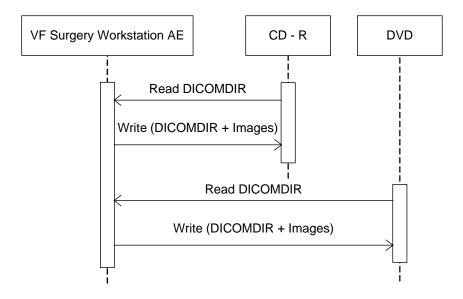
Figure 14: Sequencing of RWA Write Image
