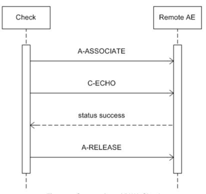
Figure 6: Sequencing of RWA Check
