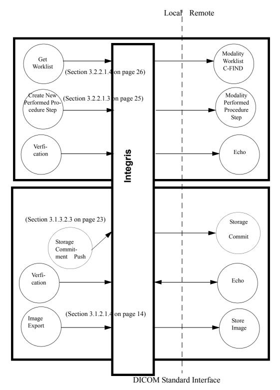
Figure 2-2: The Integris DICOM Implementation Model (with references to the related sections. Within the Integris the user interface can be used to export the images.)
