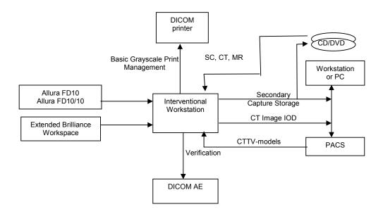
Figure 2: Interventional Workstation in a DICOM network
