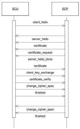
Figure 7: Message flow of TLS handshake
