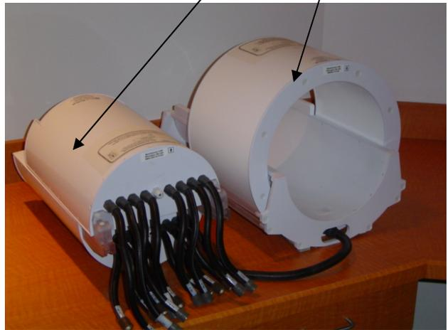
Figure 2. 7T Achieva Nova TR Coil, and Nova 16 Channel receive coil, rear view.
