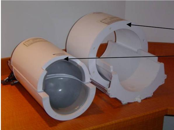
Figure 1. 7T Achieva Nova TR Coil, and Nova 16 Channel receive coil, front view
