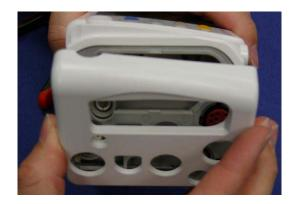
To remove the display, position the MP2 /X2 with the connectors facing towards you. Locate the heads of the two pins on the display side. Remove these by lifting them out with a screwdriver and then pulling them out manually.
