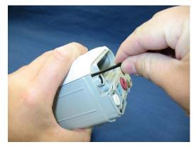
Open up the display by lifting it. The display is connected to the device with two flex cables. These flex cables are secured with two latches that open in opposite directions. The photo below shows the latches in open position.
