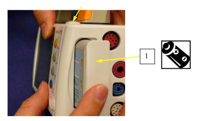
Remove the Side Cover: position the thin-bladed screwdriver in the small slot provided for this purpose. Then push off the side cover. A click signals that the cover has been removed from its position.
