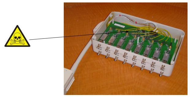
Figure 2 7T Achieva 16Channel interface box, showing circuit boards.
