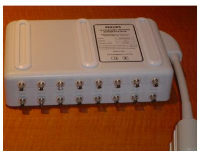
Figure 1. 7T Achieva 16 Channel Interface box.
