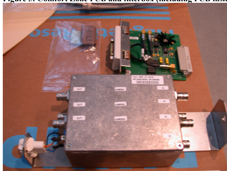
Figure 5: Comfort Zone PCB and filterbox (including PCB inside)
