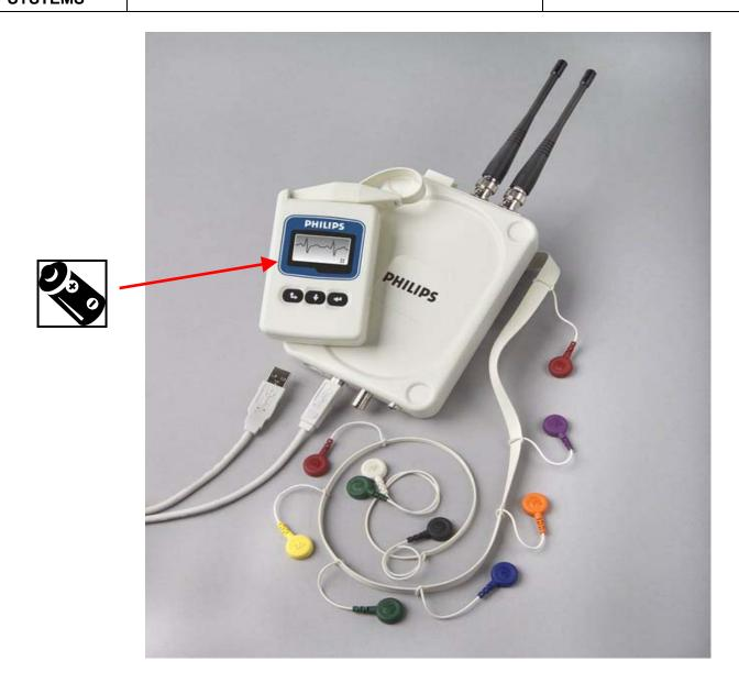
Wireless ECG Module with USB Connector: Includes AA battery see battery door on back of ECG transmitter for removal.
