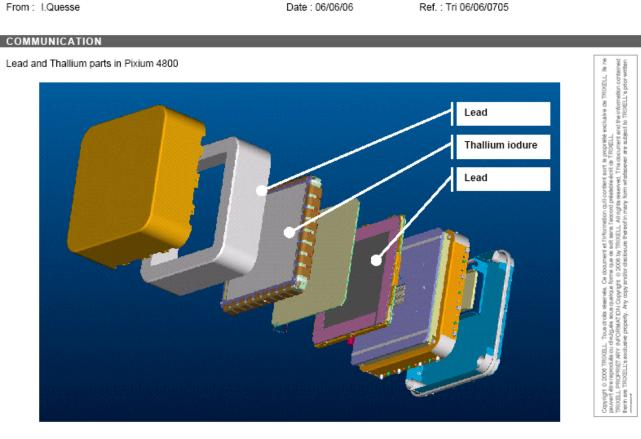
The plate just right to the utmost right lead plate is the cooling plate. This contains 58 ml **Glycoshell SF.**
