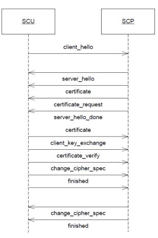
Figure 12 Message flow of TLS handshake
