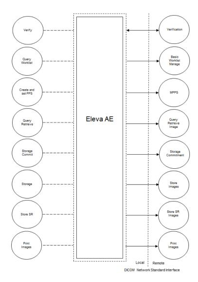
**Figure 2: Application Data Flow Diagram**
