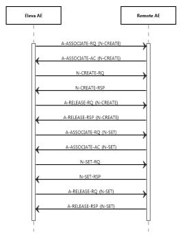
Figure 7: Modality Performed Procedure Step as SCU
