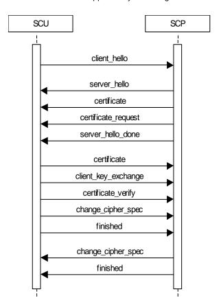
Figure 17: Message flow of TLS handshake
