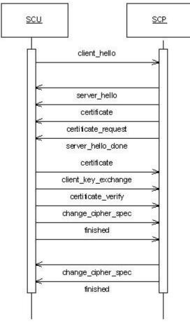
Figure 17: Message flow of TLS handshake
