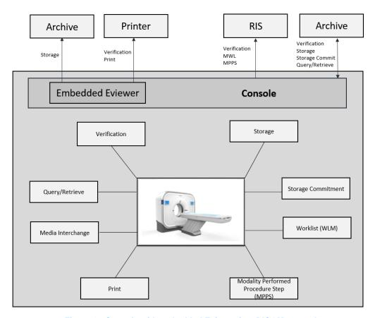
Figure 1: Console with embedded Eviewer in a DICOM network
