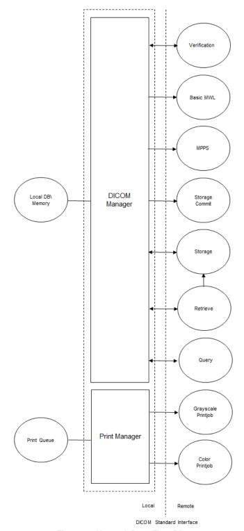
Figure 2: Network Data Flow Diagram
