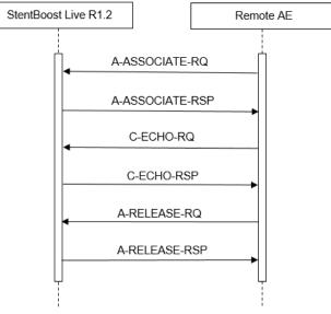
Figure 6: Data Flow Diagram – Verification as SCP
