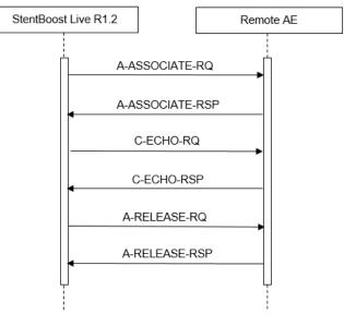
Figure 3: Data Flow Diagram – Verification as SCU
