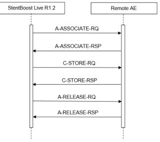
Figure 4: Data Flow Diagram – Store Image – Storage as SCU
