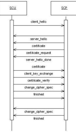
Figure 7: Message flow of TLS handshake
