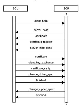
Figure 14: Message flow of TLS handshake
