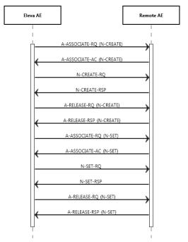
Figure 6: Modality Performed Procedure Step as SCU
