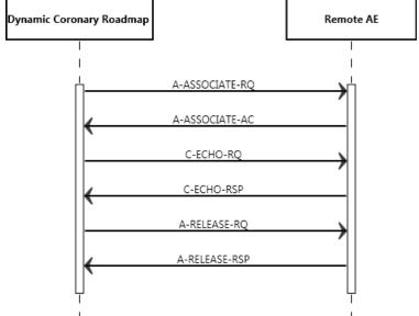
Figure 3: Data Flow Diagram – Verification as SCU
