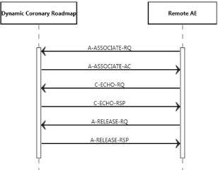
Figure 6: Data Flow Diagram - Verification as SCP
