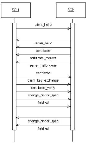
Figure 7: Message flow of TLS handshake
