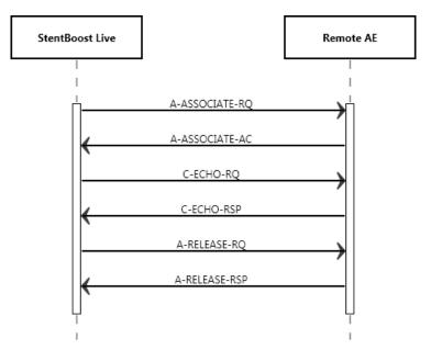
Figure 5: Data Flow Diagram – Store Image – Storage as SCU
