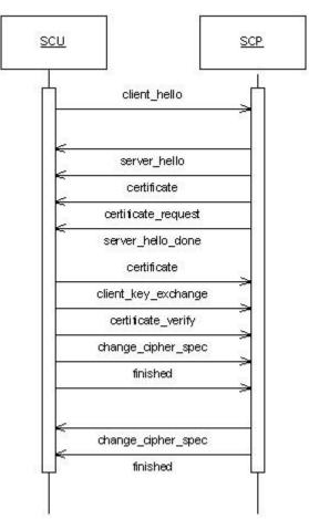
Figure 8: Message flow of TLS handshake
