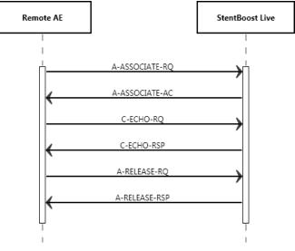
Figure 7: Data Flow Diagram – Verification as SCP
