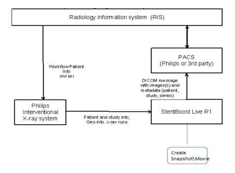
Figure 1: StentBoost Live system context regarding DICOM connectivity interfaces
