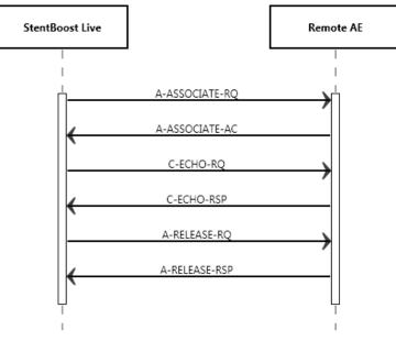
Figure 4: Data Flow Diagram – Verification as SCU
