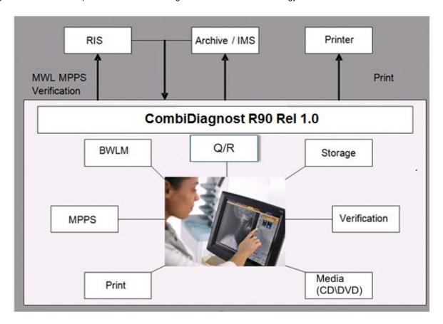
Figure 1: CombiDiagnost R90 in a DICOM network
