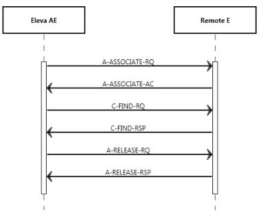
Figure 13: Data Flow Diagram - FIND as SCU
