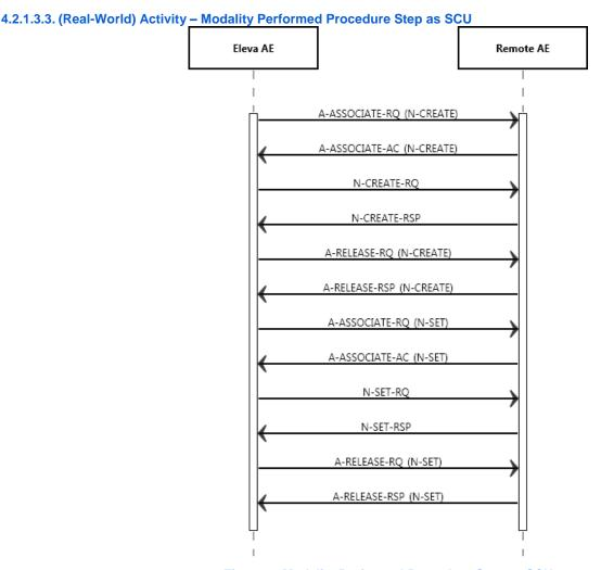
Figure 7: Modality Performed Procedure Step as SCU
