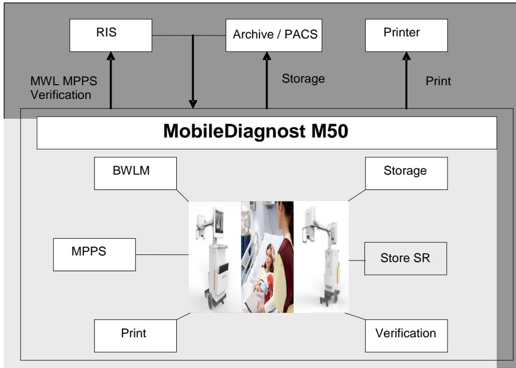
**Figure 1 MobileDiagnost M50 in a DICOM network**
