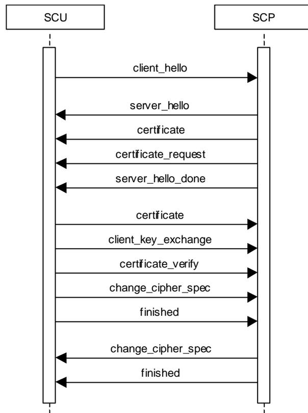
Figure 14 Message flow of TLS handshake
