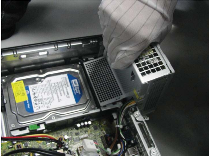
Figure 11 Remove PSU from MB
