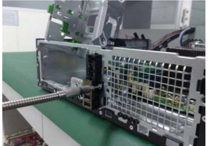
Figure 28 Loose screw of FIO and remove FIO
