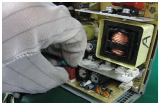
Figure 42 Remove the power supply cable from the power supply
