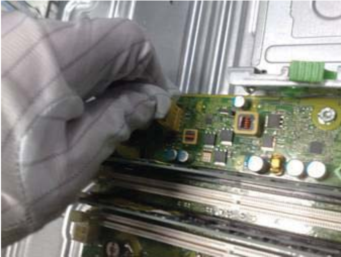
Figure 27 Disconnect FIO cables from MB
