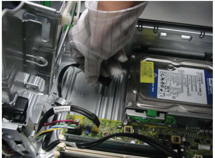
Figure 20 Remove SATA data cable from HDD
