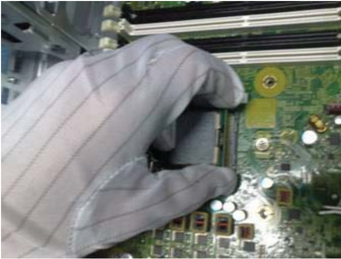
Figure 35 Loose the screws of COMB card and remove
