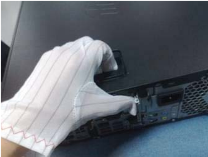
Figure 3 Disconnect the cables from fan duct
