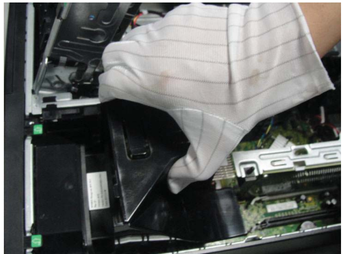
Figure 4 Remove fan duct from the board
