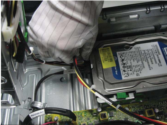
Figure 19 Remove SATA data cable from MB
