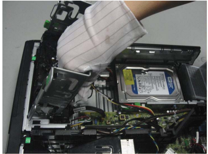
Figure 4 Remove fan duct from the board
