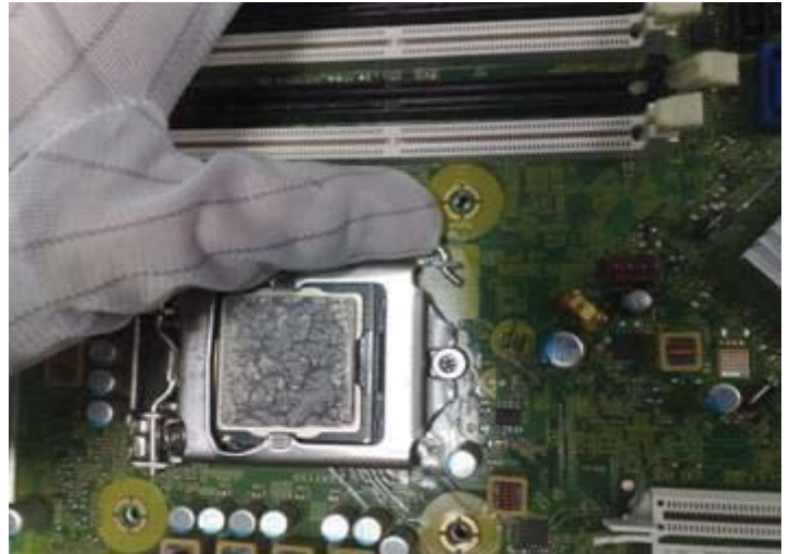
Figure 32 Rotate CPU socket handle and open it up
