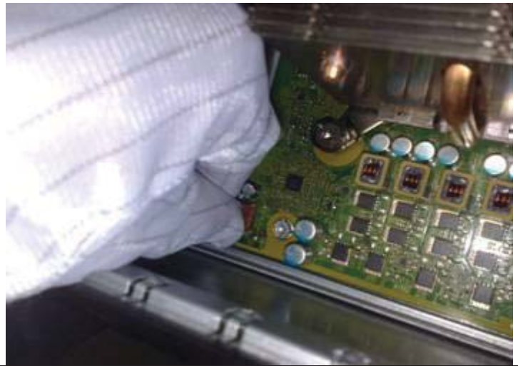
Figure 24 Disconnect front system fan cable from MB
