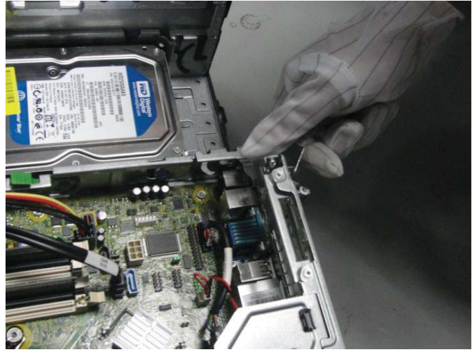
Figure 12 Loose PCI latch cover from chassis
