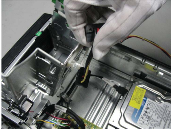
Figure 20 Remove SATA data cable from HDD
