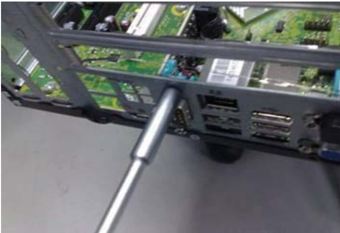
Figure 35 Loose the screws of COMB card and remove
