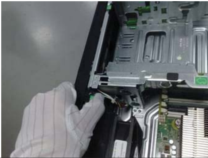
Figure 23 Remove front panel
