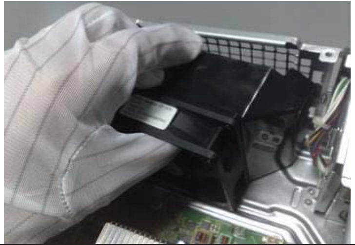
Figure 28 Loose screw of FIO and remove FIO
