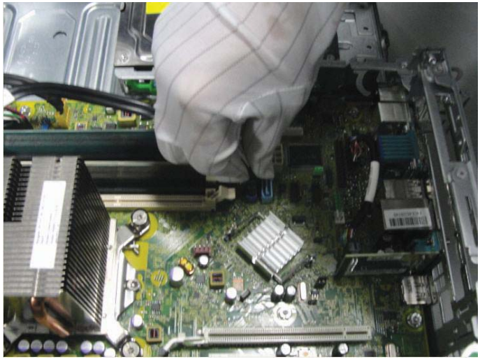
Figure 19 Remove SATA data cable from MB
