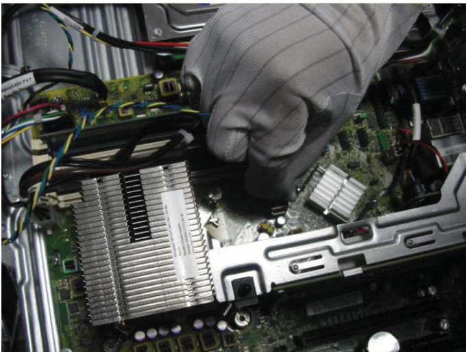
Figure 7 Disconnect front PSU fan cable from MB
