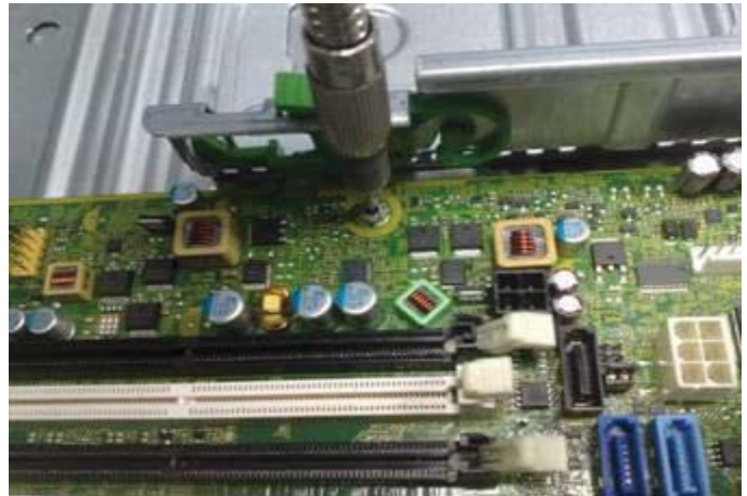
Figure 36 Loose MB screws from chassis
