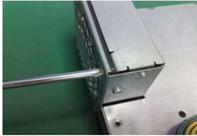
Figure 40 Remove the four screws on the board
