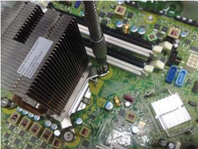
Figure 31 Loose the screws and remove heat sink
