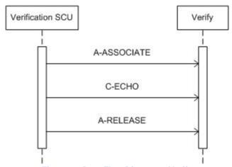
Figure 3: Data Flow Diagram - Verify
