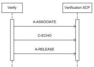
Figure 5: Data Flow Diagram - Verification as SCU
