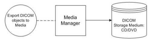
Figure 20: Media Application Data Flow Diagram
