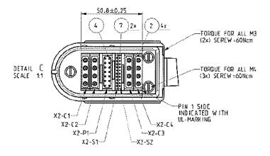
Fig 5: Layout of ODU connector
