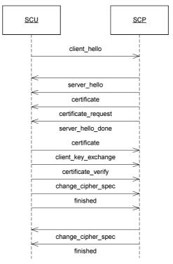
Figure 12 Message flow of TLS handshake
