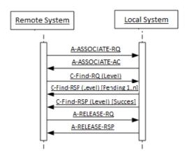
Figure 7: Data Flow Diagram - FIND as SCP
