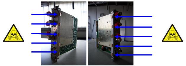
Figure 2, Berylium Sticky-Fingers on Printed circuit board assembly
