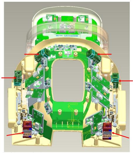
Figure 4, NVC Head Neck 3T RF trap locations
