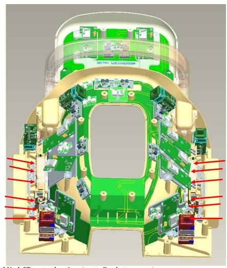
Figure 3, NVC Head Neck 3T contact locations (protruding bottom cover)
