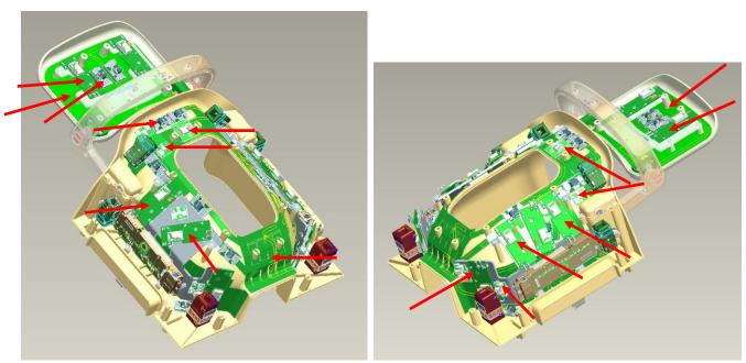
Figure 1a, 1b, NVC Head Neck 3T examples of pcb locations
